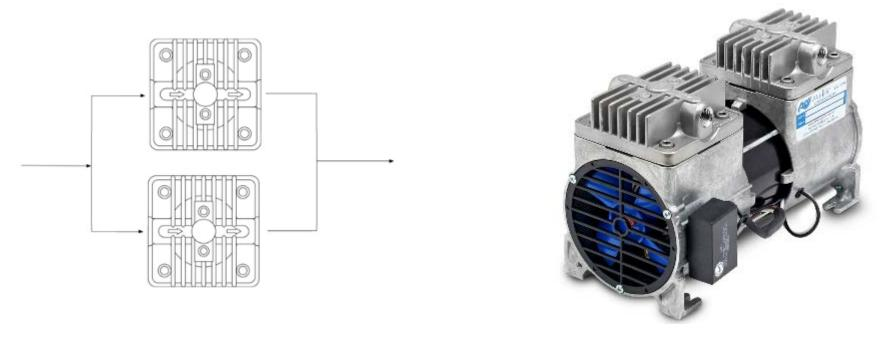
When the inlet and outlet ports of the two heads are connected in parallel, there will be continuous action at the interconnect junctions and no dead time between inlet or outlet pulses. The result of this design is smoother gas flow with greatly reduced pulsation effects at the inlet and outlet connections; in addition, sample line pressure losses are correspondingly reduced because of the reduced peaked and nearly-constant flow rate.
