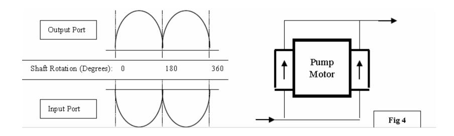
When the inlet and outlet ports of the two heads are connected in parallel, there will be continuous action at the interconnect junctions and no dead time between inlet or outlet pulses. The result of this design is smoother gas flow with greatly reduced pulsation effects at the inlet and outlet connections; in addition, sample line pressure losses are correspondingly reduced because of the reduced peaked and nearly-constant flow rate.
