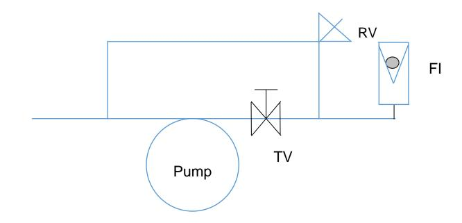
Relief valve reduces high pressure pulses on pump diaphragm, flow pulses will be reduced; return line may be connected to process or pump inlet. (Lowest Cost)
