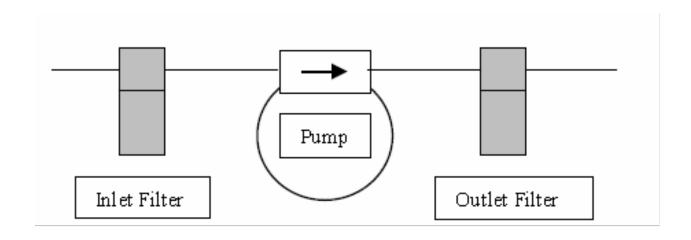
Addition of a filter at the inlet & outlet will reduce the **pump outlet** pressure pulse amplitude. This is important when flowmeters or other pressure-sensitive instrumentation is used, as pulsation will give false readings.
