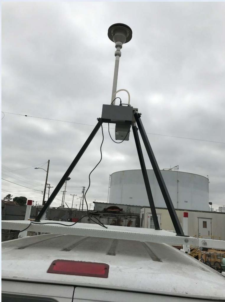
PQ 100 Sampler - Sampling for Cr(VI) typically involves collecting a sample on a filter and having this filter analyzed at a qualified lab. The filter and cassette are obtained from the lab and a small sample pump is used to pull air over the filter for a specified amount of time at a controlled rate. SCAQMD collect filter media every 3 days for lab analysis.
